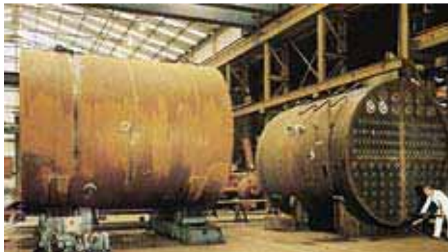
A typical waste heat boiler of the shell and tube pattern under construction. Note that there is no combustion chamber, only tubes.
